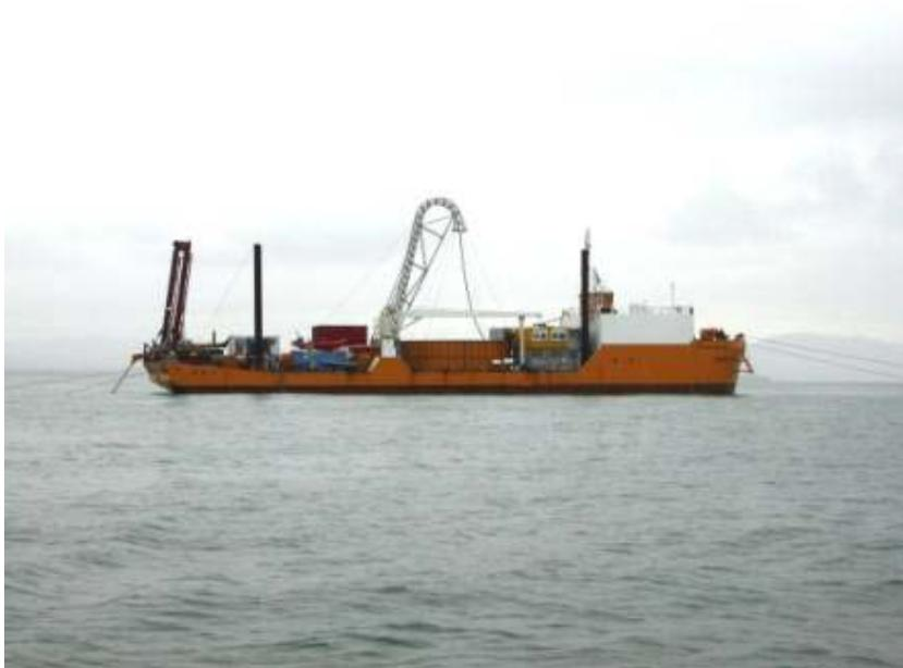
Illustration: Cable laying vessel
